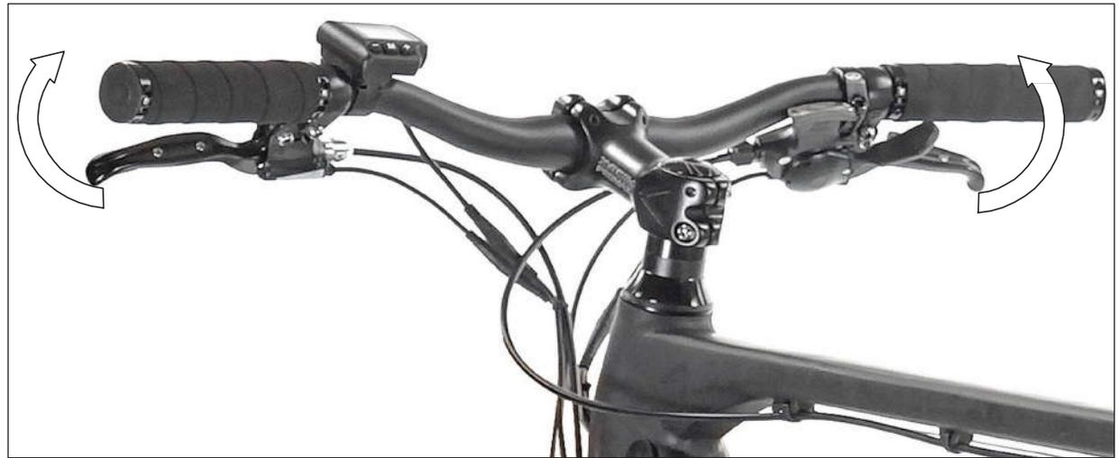
Handbrake lever for front brake
