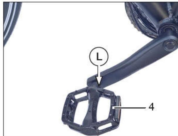
Check regularly if the pedals(4) are screwed firmly on the cranks.
