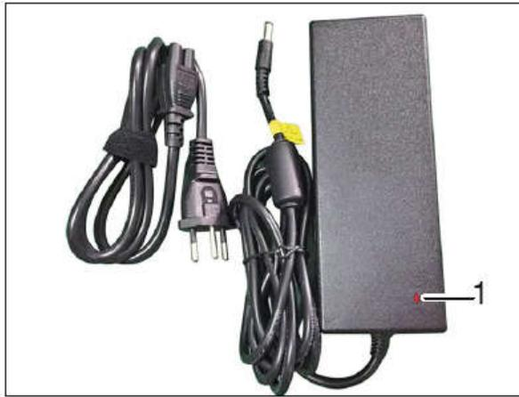
This charger is suitable for Li-ion batteries. The LED (LED 1) on the charger keeps you constantly informed of the operating status. You will be informed about the status and charging of the battery at a glance.
