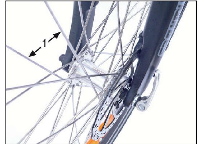
A tight fit of the spokes (1) is for the Impact-free running of the wheels important. loose
