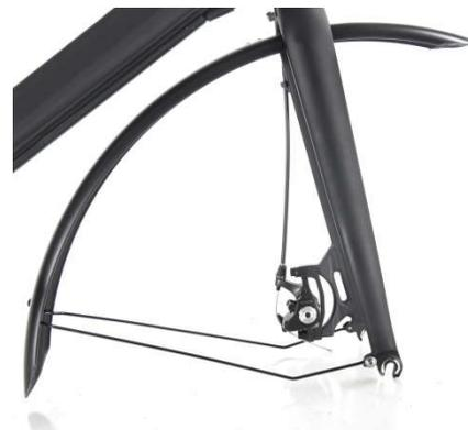
4. Fix the front disc brakes with the inner six screws on the front fork disc brake mount. There are two installation methods: radial mounting and axial mounting..
