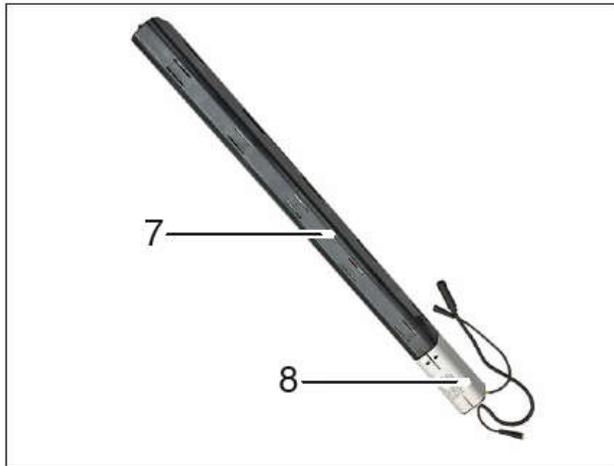
Disconnect the battery (7) and controller (8)
