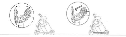
If your standpipe in electric scooter is shaking, please use the M5 hex wrench to lock the two screws at the fold mechanism.
