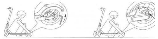
If you feel the brakes are too tight, please use the M5 hex wrench counterclockwise to release the pressure plate screws on the disc brake seat, return the brake line to make the exposed tail length slightly shorter, and lock the pressure plate screws; If you feel the brake is too lose, release the
