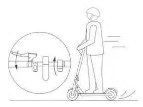
4.Release the throttle finger can slow deceleration, energy recovery system automatically open to help slow down, emergency brake need to shake the brake,handle at the front left handle.
