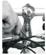
Hexagon socket screw (integrated stop notch)
