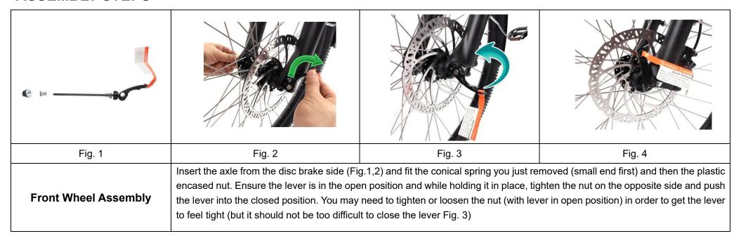
WARNNING: IT IS IMPERATIVE THAT THE QUICK RELEASE IS SECURELY TIGHTENED AND PROPERLY ALIGNED, TO PREVENT THE WHEEL FROM COMING OFF, CAUSING DAMAGE TO THE BIKE OR SERIOUS INJURY.
